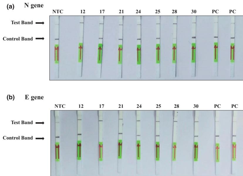
**FIGURE 4** Representative lateral flow readouts from patient samples. Lateral flow readout results from patient samples of N (a) and E (b) genes for one NTC, seven PS (Ct values 12, 17, 21, 24, 25, 28 and 30) and two PC (Ct values >33) after 3 min. PC, patient control; PS, patient samples
