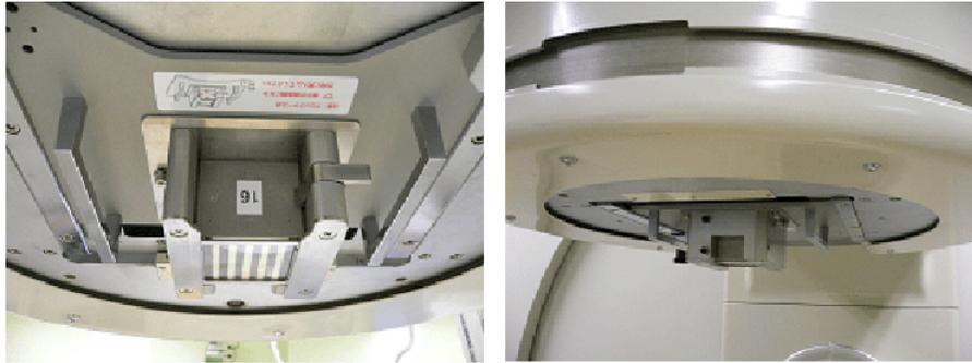
FIG. 2. Photographs of the cubic-block-piled compensator mounted on the accessory mount of the linear accelerator gantry head.
