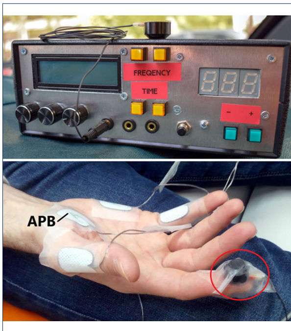
Figure 1. Vibration stimulator with tactor on the upper extremity digit II, and surface electrodes over the abductor pollicis-brevis (APB) muscle. Top: Custom made vibration stimulator (upper). Bottom: The position of the tactor, a miniature electromagnetic solenoid-type stimulator (Dancer Design, St. Helens WA10 1 LX, UK), on digit II with surface electrodes (encircled in red) attached over the APB muscle.
