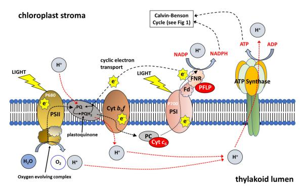
**Figure 2.** Schematic Representation of Photosynthetic Electron Transport. Photosystem I (PSI), Photosystem II (PSII), Cytochrome b6f complex (Cyt  $b_6f$ ), plastocyanin (PC), Ferredoxin (Fd) and ferredoxin-NADP reductase (FNR). Cytochrome  $c_6$  (Cyt  $c_6$ ) transfers electrons from the Cyt  $b_6f$  complex to PSI at a faster rate than observed for PC; plant ferrodoxin-like protein (PFLP) (Adapted from [23]).
