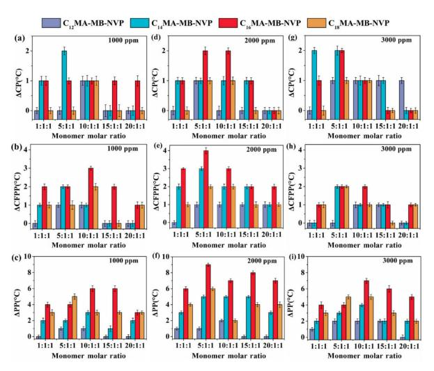
**Figure 12.** Effects of 1000 ppm (**a**–**c**), 2000 ppm (**d**–**f**), and 3000 ppm (**g**–**i**) RMC-BM-NVP terpolymers on  $\Delta$ CP,  $\Delta$ CFPP, and  $\Delta$ PP of B20 (RMCMB-NVP = methacrylate-benzyl methacrylate-*N*-vinyl-2-pyrrolidone terpolymers, R = C12, C14, C16, C18). Reprinted with permission from [161]. Copyright (2020) Wiley-VCH Verlag GmbH & Co.
