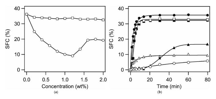
**Figure 7.** (a) Solid Fat Content (SFC) NMR analysis for PGE and EVA additives (2 wt%, open circles and open squares, respectively) taken at 9 °C after 60 min; (b) Time variation of SFC with and without additives measured at 9 °C. Pure PFME (closed circles), 1 wt% EVA (open squares), 2 wt% EVA (closed squares), 1 wt% PGE (open triangles), 2 wt% PGE (closed triangles) and 1 wt% PGE + 1 wt% EVA (open circles). Reprinted with permission from [127]. Copyright (2010) Wiley-VCH Verlag GmbH & Co.
