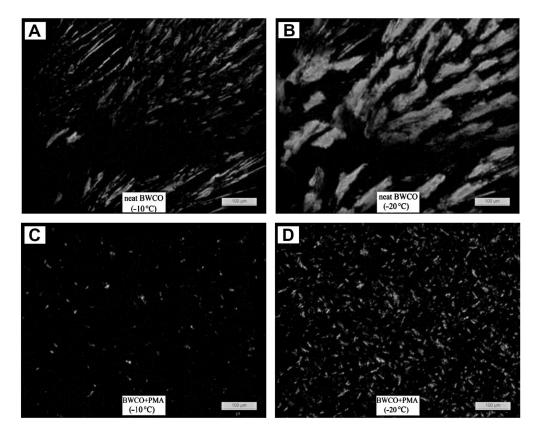
**Figure 9.** Polarizing optical microscopy images of crystal morphologies of waste cooking oil BD without or with polymethyl acrylate: crystallization of saturated FAMEs without additive at  $-10 \degree C$  (**A**) and  $-20 \degree C$  (**B**), and with additive at  $-10 \degree C$  (**C**) and  $-20 \degree C$  (**D**). Reprinted with permission from [98]. Copyright (2014) Elsevier B.V.
