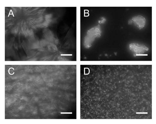
addition of 1 wt% EVA copolymer and 1 wt% PGE caused the formation of small crystals (Figure 8D). For the last case, CFPP was reduced by the value of 6  $^{\circ}$ C.
