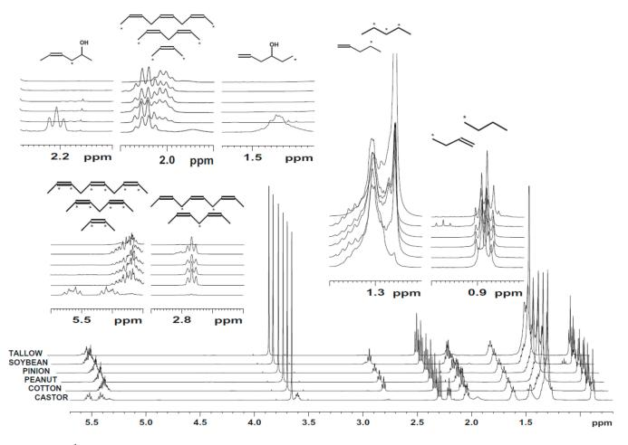
**Figure 6.** <sup>1</sup>H NMR spectra for pure biodiesel samples from different sources. Reprinted with permission from [82]. Copyright (2012) Elsevier B.V.
