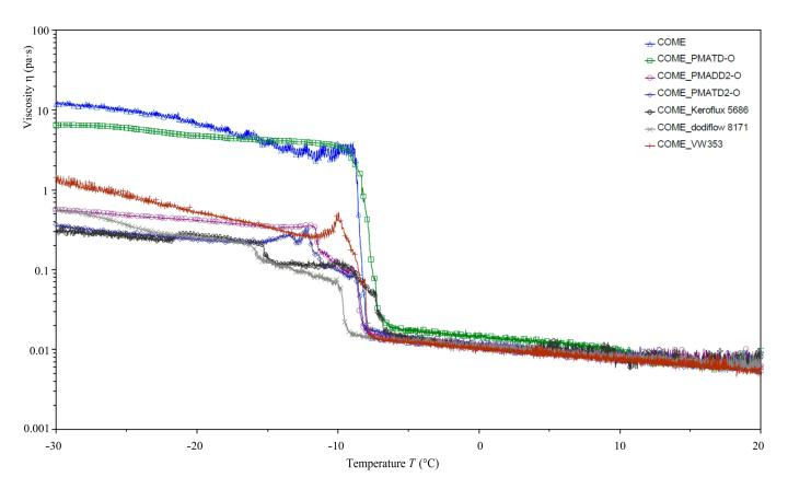
**Figure 11.** Viscosity vs. temperature curves for corn oil biodiesel (corn oil methyl esters, COME) and COME containing 0.1 wt% polymer additives. Reprinted with permission from [152]. Copyright (2021) Elsevier B.V.
