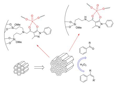
**Figure 7.** Sketch of the general procedure for the preparation of SBA-15 anchored oxidovanadium based catalysts.
