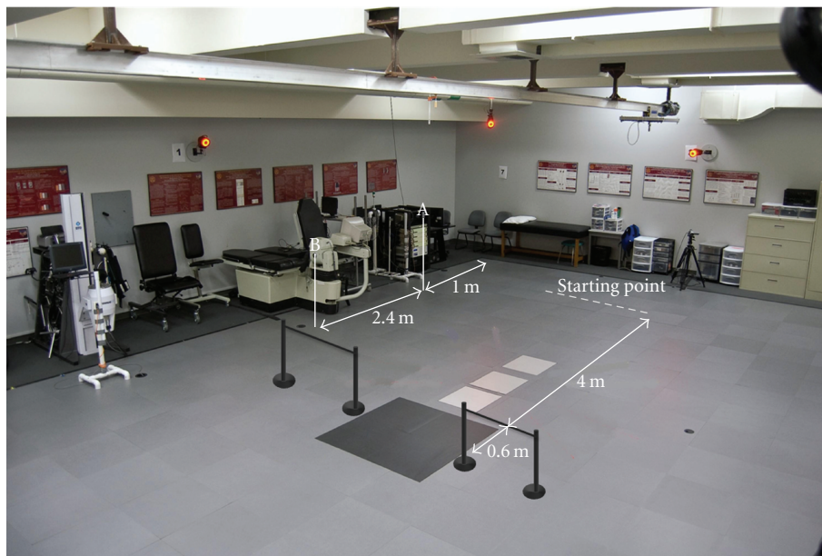
FIGURE 1: Laboratory setup. Dashed line: starting point; A: first trigger; B: second trigger; black square: force plate (AMTI 1.2 m × 1.2 m, 1560 Hz). Two stanchions were placed at the midpoint of each force plate. Starting point to A: 1 m. A to B: 2.4 m. B to force plate: 0.6 m. Force plate to stanchions: 0.6 m.
