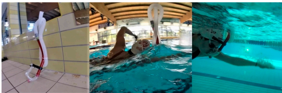
Figure 1. An instrument increasing added respiratory dead space: a custom added respiratory dead space (ARDS) apparatus consisting of a polypropylene centre-mount swimming snorkel with a mouthpiece (Speedo International Ltd., Nottingham, UK) integrated with 2.5-cm diameter ribbed tubing to provide 1000 mL of dead space.
