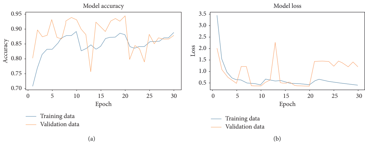
FIGURE 7: Inception-ResNetV2 model accuracy and model loss for each epoch. (a) Accuracy vs. epoch. (b) Loss vs. epoch.
