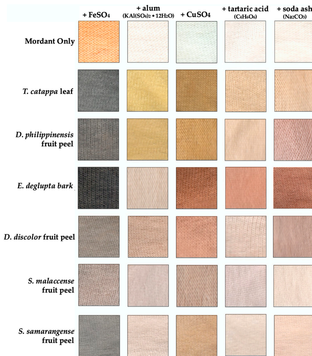
Figure 3. Color palette from the biowaste dyes applied in cotton using different mordants. Comparison of color is through the measured hue (color component), value (lightness), and saturation (intensity). Lighter color (low %V value) is obtained in the presence of FeSO 4 , especially for E. deglupta and T. catappa (both black). D. philippinensis extract mordanted with alum also produced yellow comparable to the well-studied T. catappa . Interestingly, red-brown coloration was uniquely observed in E. deglupta with CuSO 4 or alkali.
