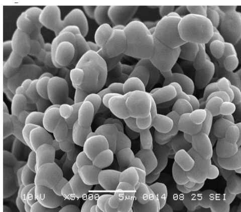
Figure 3. Representative scanning electron microscope (SEM) image of milled isoniazid without excipients. B2 batch. Magnification: 5000×.
