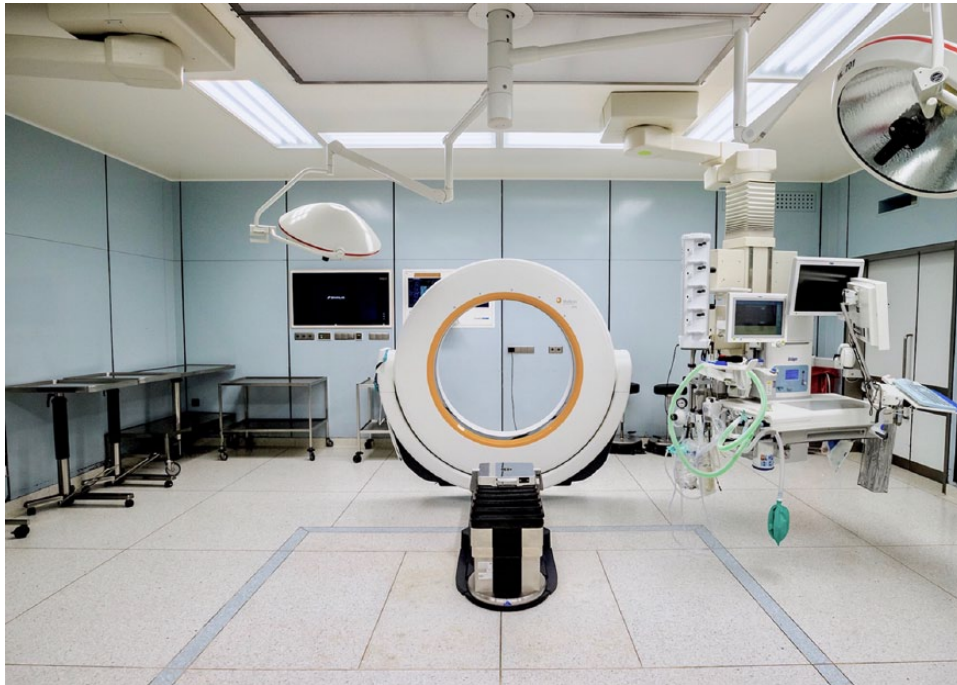
Fig. 8 Mobile intra-operative CT Brainlab Airo®.
