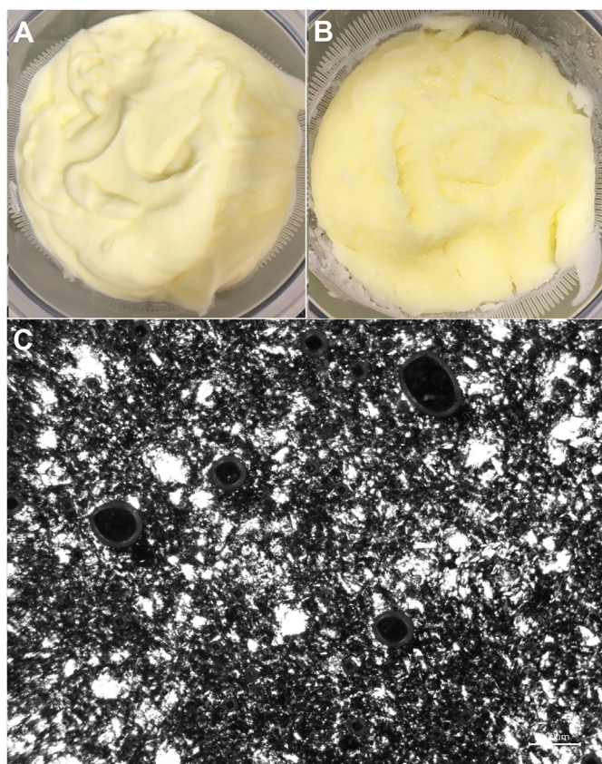
Fig. 5. Images of an experimental margarine sample prepared with tignut glycerolysis product (A) 1 week and (B) 10 months after sample preparation. Sample was stored at 5 °C in both cases. (C) Microstructure of the tignut glycerolysis product margarine after 10 months storage at 5 °C.
