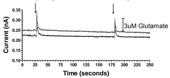
Each tail pinch evoked an immediate increase in the current corresponding to glutamate concentration changes of 2.9  $\mu$ M and 4.9  $\mu$ M at the two electrode sites. Not surprisingly, these are much smaller responses than produced by the high intensity, high frequency stimulation described above but, similar to the electrical stimulation data, subsequent tail pinches resulted in approximately a
