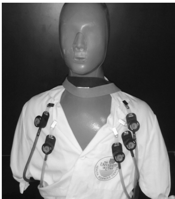
Figure 5. IOM sampler setup on a rotating mannequin in a low speed wind tunnel.
