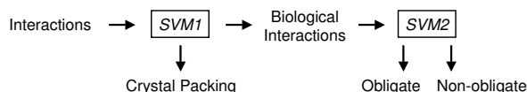
Figure 1 Schematic plot of the two-stage SVM. If an interaction is classified as crystal packing by SVM1, it will not be considered by SVM2; otherwise it is classified by SVM2 as either obligat or non-obligat interaction.
