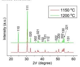
**Figure 2.** XRD patterns for annealed ZST Samples A and B (Table 1) obtained for sintering temperatures of 1150 °C and 1200 °C, respectively.
