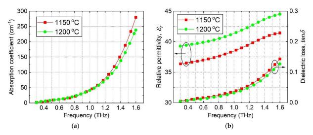
**Figure 4.** Frequency dependence of (a) the absorption coefficient, and (b) relative permittivity and the dielectric loss tangent versus sintering temperature for ZST ceramics (Samples A and B were sintered at 1150 °C and 1200 °C, respectively).
