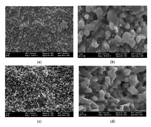
**Figure 3.** SEM micrographs of the ZST samples sintered at  $(\mathbf{a},\mathbf{b})$  1150 °C and  $(\mathbf{c},\mathbf{d})$  1200 °C. The images were recorded at  $(\mathbf{a},\mathbf{c})$  5000× magnification and  $(\mathbf{b},\mathbf{d})$  25,000× magnification using an accelerating voltage (EHT) of 20 kV.
