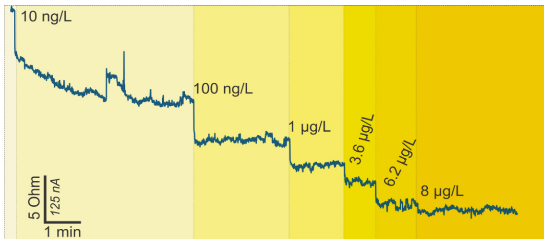
Figure 3. Change in resistance versus time readings for the GFET ferritin biosensor on the addition of ferritin-free buffer (phosphate-buffered saline (PBS)) and increasing ferritin concentration.
