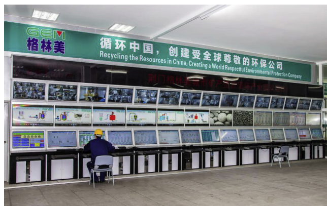
Fig. 5. The automatic control system of GEM power battery precursor material production line. [Photo courtesy of GEM Co., kindly reproduced from gem.com.cn].
