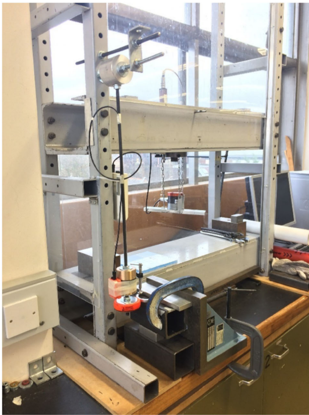
FIGURE 1. Image (left) and a schematic (right) of the pendulum test rig. A mass ( m ) and an accelerometer ( a ) are mounted directly above the impactor ( i ) to reproduce ball impact in hockey games. The electronic component, a light-emitting diode (LED) is mounted directly on the dental model, on which the mouthguard is mounted.
