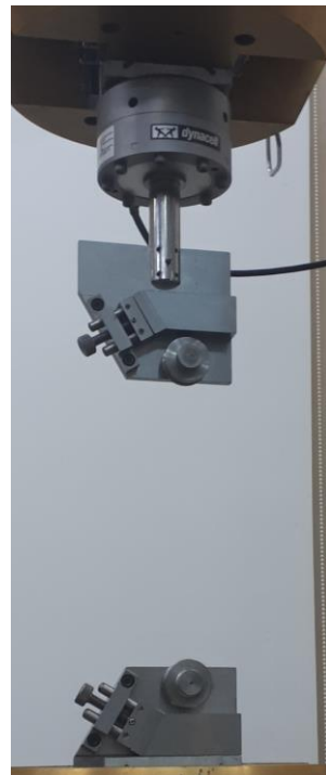
Figure 4. Thread grips installed in the hydraulic clamps of the testing machine with an additionally installed force precise measuring head.
