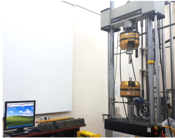
Figure 5. Instron 8802 testing machine for static tests.
