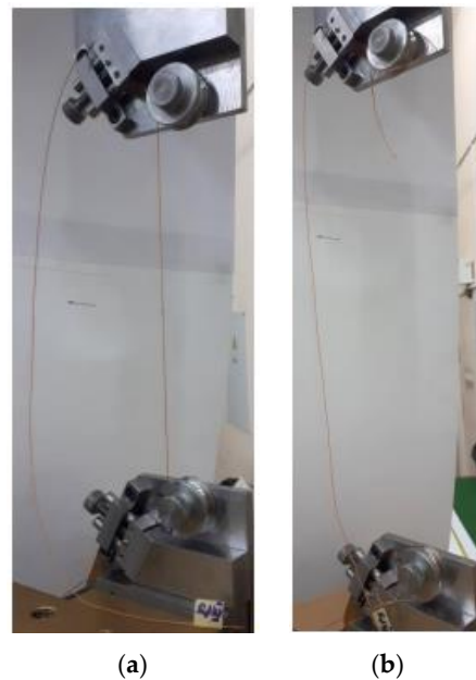
Figure 7. Photos of tested sample of cord III: (a) before test and (b) after test.
