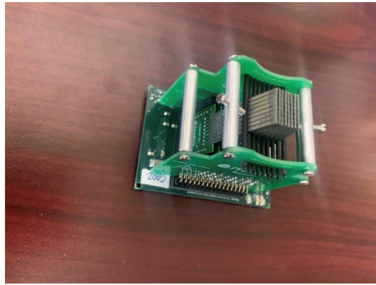
Figure 1. A photo of the Latero device without the external plastic cover. On the top of the device is an array of 8 \times 8 pins, where participants place their fingertips to feel the tactile vibration.
