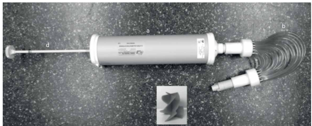
FIGURE 1 Physical lung model composed of a) a 3 L Hans Rudolph syringe, b) an attachment made from 18 flexible tubes, c) a helical mixer device inserted at the syringe entrance, and d) an adjustable syringe stopper.
