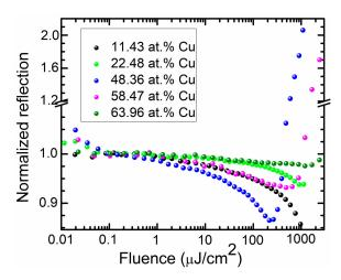
Figure 9. The normalized reflectance vs laser fluence for the selected hydrogen-free DLC:Cu films.
