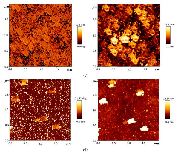
**Figure 4.** Atomic force microscopy (AFM) images of DLC:Cu samples containing different amount of copper: 22.48 at.% Cu (a), 32.45 at.% Cu (b), 48.36 at.% Cu (c), 58.47 at.% Cu (d). Phase images are presented at the left and morphology images are at the right.
