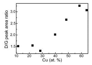
Figure 7. D/G peak area ratio Vs copper atomic concentration in DLC:Cu films.
