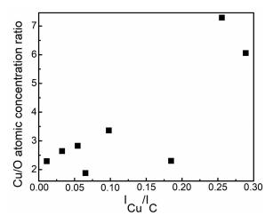
**Figure 2.** Copper and oxygen (Cu/O) atomic concentration ratio Vs copper and carbon target current ratio ( $I_{Cu}/I_{C}$ ). Atomic concentrations measured after the *In situ* ion beam etching were analysed.
