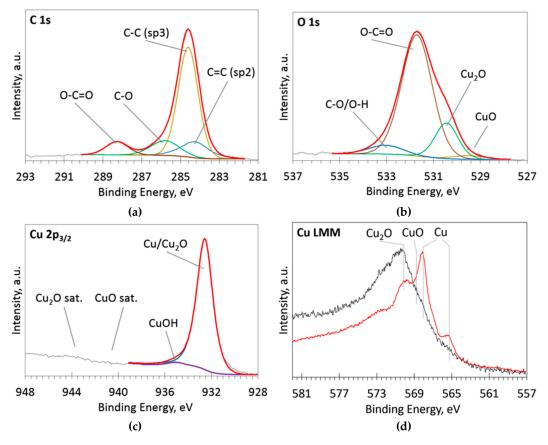
**Figure 3.** Deconvoluted high resolution C1s (a), O1s (b), Cu2p (c), Cu LMM (d) X-ray photoelectron spectra (XPS) spectra of the sample Cu09. Black thin line–acquired data, colored thick lines—fitted peaks, red thick line—envelope.
