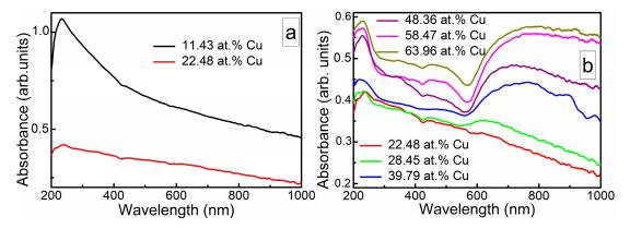
Figure 8. The representative optical absorbance spectra of DLC:Cu films:  $\leq$ 22.48 at.% Cu, disappearance of diamond like carbon (DLC) related absorption peak at lower wavelengths (a);  $\geq$ 22.48 at.% Cu, rise of the plasmonic peak (b). Absolute absorbance values are adjusted to make their analysis easier. The absorbance curves were lined up according to the Cu amount in the films in (b).
