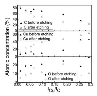
Figure 1. Chemical composition of DLC:Cu films Vs copper and carbon target current ratio.
