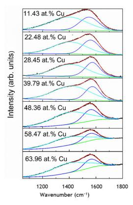
Figure 6. The representative Raman scattering spectra of hydrogen-free DLC:Cu films.
