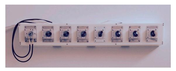
**Figure 4.** Peristaltic pump array permitting every flask to be connected to the central receiving flask from which every other flask can be reached. The Viton tubing is shown connected only to the left-most pump and the wiring connecting the pump array to the custom programmable electronic control box is visible at the extreme left.
