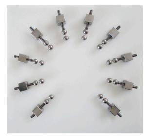
Figure 7. Arrangement of the custom Marx generator showing the spark gap electrodes, which permit the spark gap distance to be varied by means of a threaded screw arrangement.
