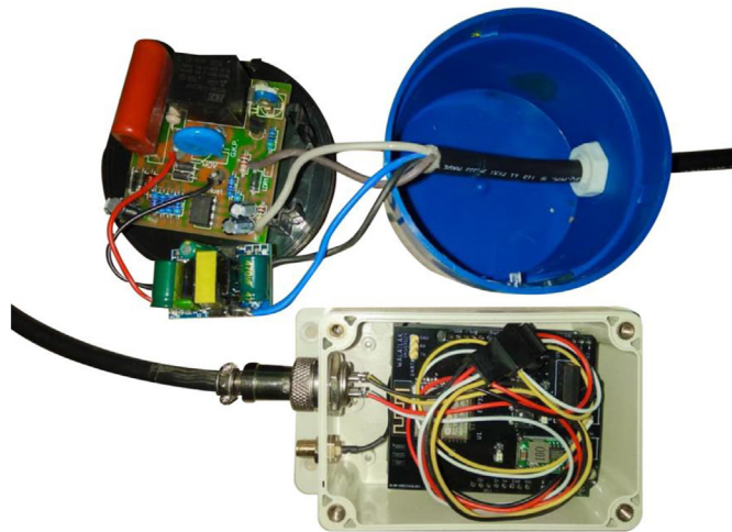
Figure 5. An SLCB unit is constructed of two boxes connected by four-core cables. The round box includes the modified photo switch module, which will be connected to the relay unit. The square box contains the microcontroller and NB-IoT modules. This box will be placed in the electrical control case of the traditional street lighting system. An antenna will be mounted externally to receive the full signal.
