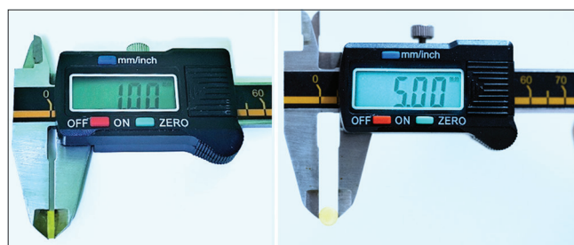
Figure 1: The bonding agent discs after removal from the mould confirming the dimensions (thickness and diameter) of the bonding agents discs
