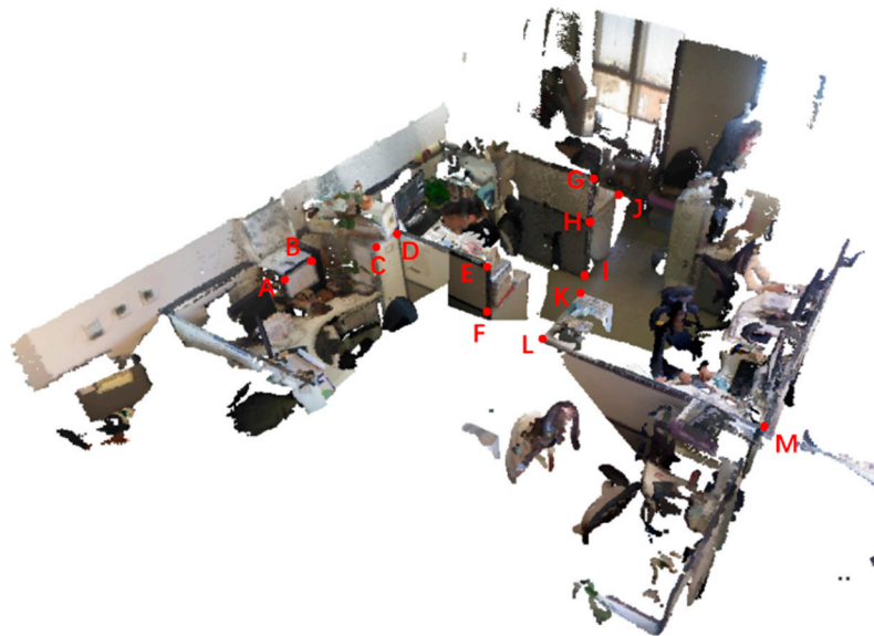
Figure 8. 3D reconstruction result by our method and the measured points. A–M are the end points of line segments.
