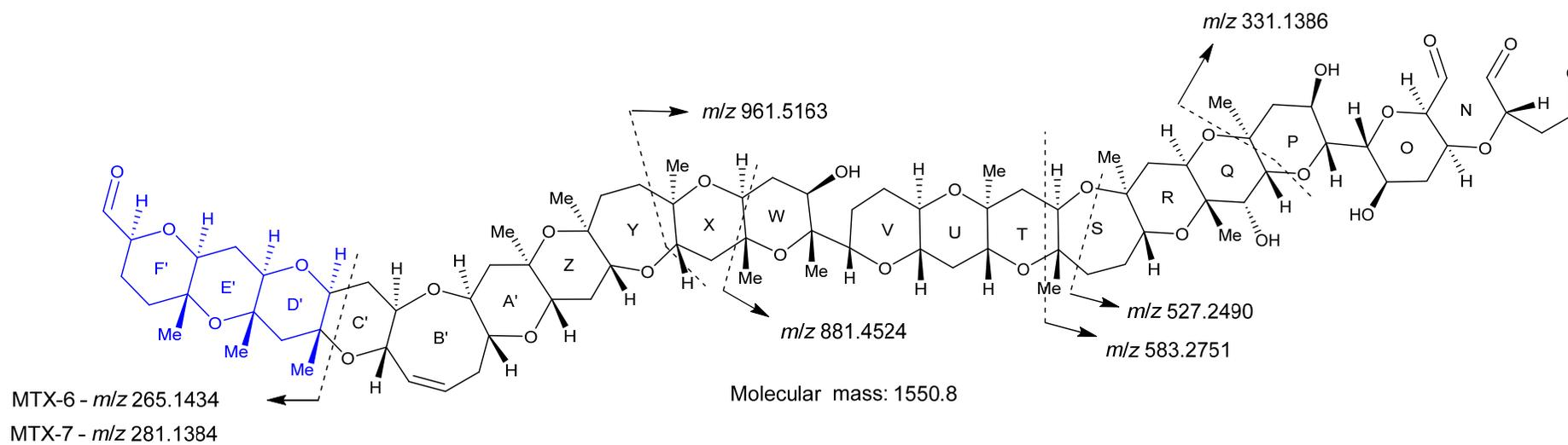
**Figure 5.** Proposed CID fragmentation pathway for the truncated 'Fragment B' of MTX-6 and MTX-7, based on the chemical structure of MTX-1, showing the common fragment ions produced under collision-induced dissociation. The highlighted region (in blue) is where the additional oxygen atom in MTX-7 is likely located.
