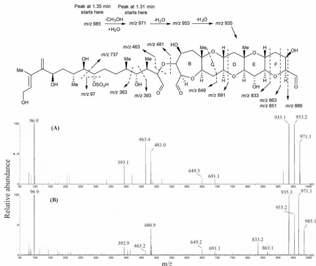
**Figure 4.** The proposed CID fragmentation of Fragment A in  $-$ ESI (60 eV CE;  $m/z$  50–1000) and comparison of the corresponding spectra of (A) MTX-1 and (B) MTX-7.
