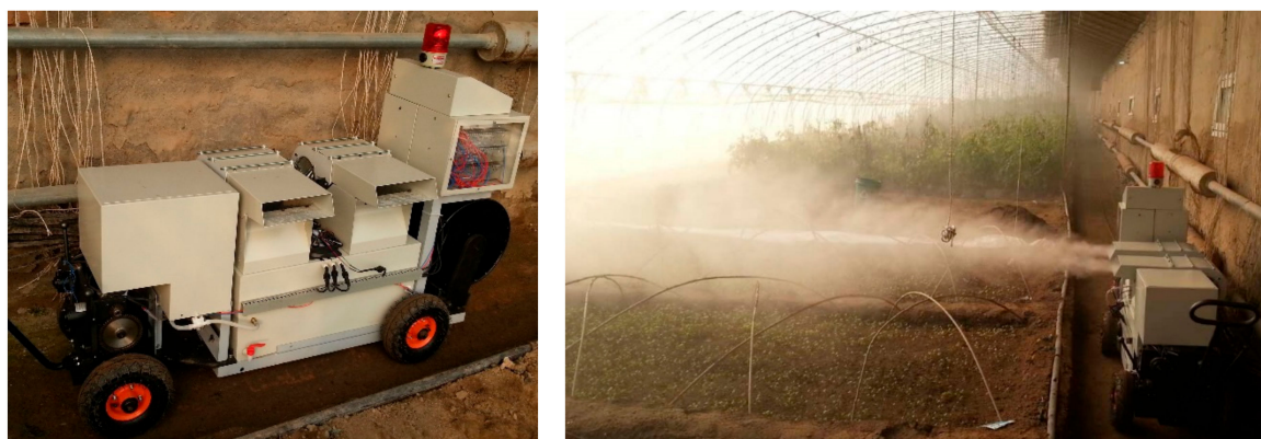
Figure 1. The self-propelled high-energy ultrasonic atomizer used in the tests.
