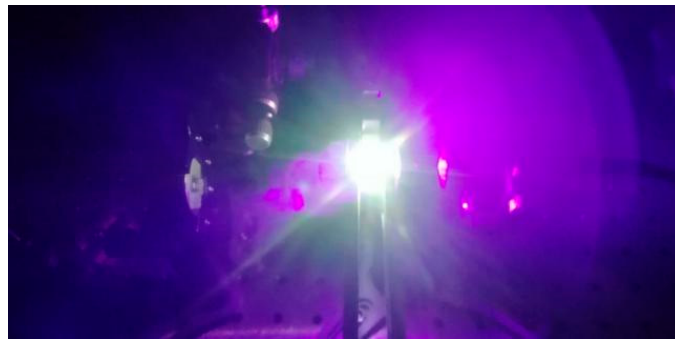
Figure 6. Harsh white light photograph of \text{Yb}^{2+} -doped glass with an excitation of 405 nm.
