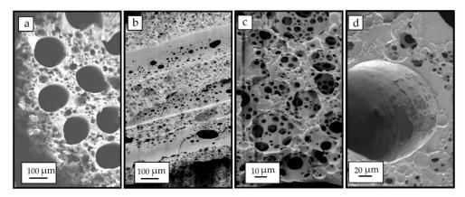
**Figure 7.** SEM images showing the transversal sections of the conduit showing the high-volume porosity created by high internal phase emulsion (HIPE) (**a**). Lumen of the microchannels after being cut and inspected by SEM, in which a high porous structure is observed (**b**), Detail of the porous structure of the manufactured implant (**c**), and detailed image of a single microchannel (**d**).
