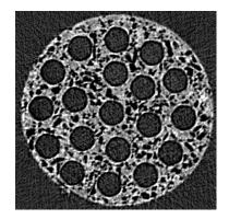
**Figure 6.** MicroCT image showing the transversal section at the middle of a 5 mm length implant containing microchannels of 200  $\mu$ m.
