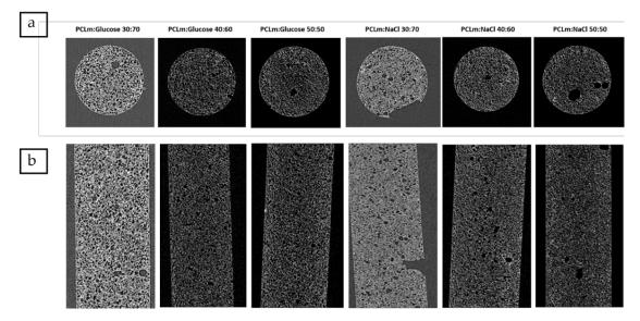
**Figure 5.** Micro computed tomography (MicroCT) analysis following different orientations: (a) transversal section and (b) longitudinal section of leached methacrylated poly- $\varepsilon$ -caprolactone (PCL) (PCLm) UV cast cylinders mixed with different percentages of porogens (sodium chloride or glucose). The tubular structures shown are all 1.5 mm diameter and 5 mm in length.
