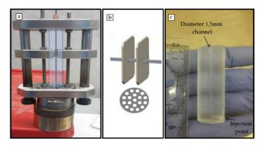
**Figure 1.** (a) Mechanical optimized setup for the 3D conduits fabrication in which the dashed line shows the position of the polydimethylsiloxane (PDMS) container. (b) Computer Aided Design (CAD) image showing distribution of the 200  $\mu$ m wires arrangement through two opposite aligned micro perforated plates. (c) PDMS container.
