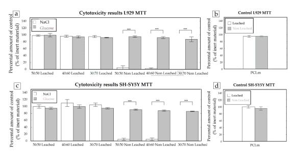
**Figure 10.** The cytotoxicity results using NaCl or glucose as porogens on PCLm conduits (n = 5). Cytotoxicity assays were performed with L929 (**a**) and SH-SY5Y (**c**) cells. As a control, PCLm cylinders were included without porogen treatment (n = 1) but, in every other way, treated the same (**b** and **d**).
