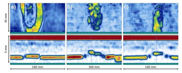
**Figure 13.** Images of samples after a lightning strike and ultrasonic tests for (**a**) L\_ref, (**b**) L\_TP and (**c**) L\_ECF, where C-Scan (top) and B-Scan (bottom) visualization.
