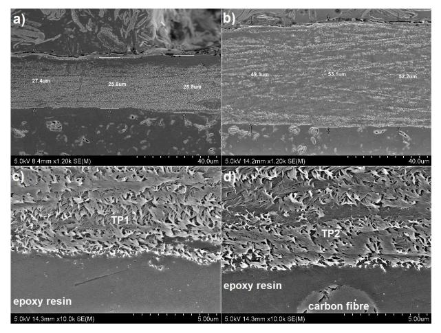
**Figure 8.** Microstructure of the cross-section of laminates with Tuball paper on the top: (**a**) and (**c**)—L2; (**b**) and (**d**)—L3. The arrow shows epoxy resin inside the layer.
