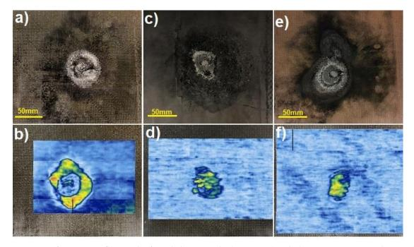
**Figure 12.** Images of composites flat panels after a lightning strike (upper row) and ultrasonic C-Scan visualization (lower row) for: (**a**,**b**) L\_ref, (**c**,**d**) L\_TP and (**e**,**f**) L\_ECF.
