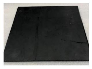
Figure 3. Test panel with Tuball paper (L\_TP). Dimensions: 300 mm  $\times$  300 mm.
