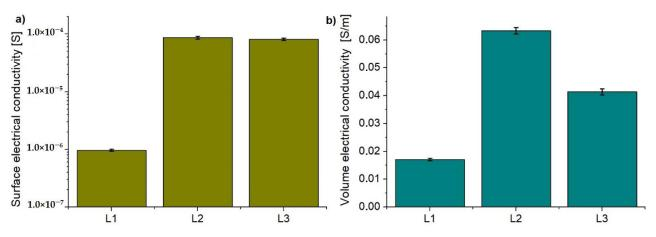
Figure 6. Electrical conductivity of CFRP panels: (a) surface, (b) Z-direction (through the thickness).
