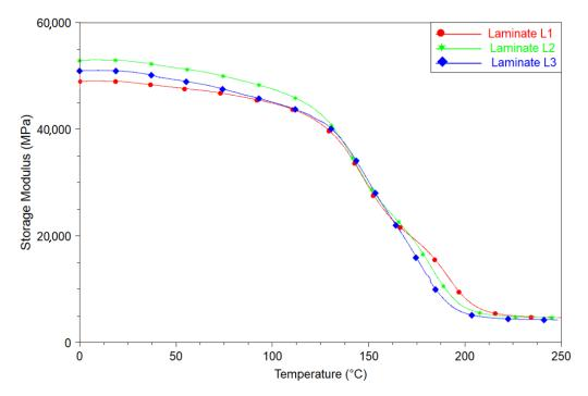
Figure 11. Storage modulus of reference (L1) and modified (L2, L3) laminates.
