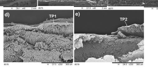
Figure 10. Microstructure of laminates after impact tests: (a) L1, (b,d) L2, (c,e) L3.
