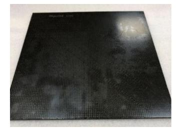
Figure 2. Reference test panel (L\_ref). Dimensions:  $300 \text{ mm} \times 300 \text{ mm}$ .
