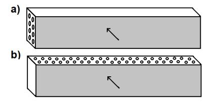
**Figure 1.** Method of performing impact resistance tests, striking edge (**a**) perpendicular and (**b**) parallel to carbon fibres.
