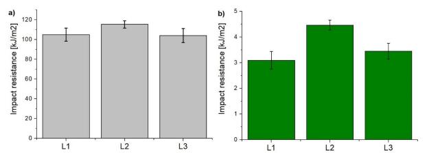
Figure 9. Impact resistance of analyzed laminates (a) perpendicular and (b) parallel to carbon fibres.
