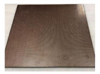
**Figure 4.** Test panel with ECF (L\_ECF). Dimensions: 300 mm  $\times$  300 mm.
