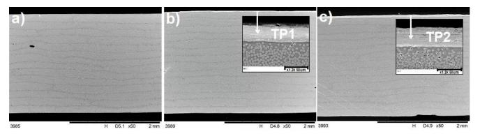
Figure 7. Microstructure of laminates cross-section: (a) L1, (b) L2, (c) L3. Arrows show the layer of Tuball paper.
