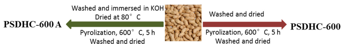
Scheme 8. Synthesis procedure of porous PSDHC-600 (peanut shell derived hard carbon obtained by pyrolysis at 600 °C) and porous PSDHC-600 A (peanut shell derived hard carbon obtained by pyrolysis at 600 °C, previously treated with KOH solution).
