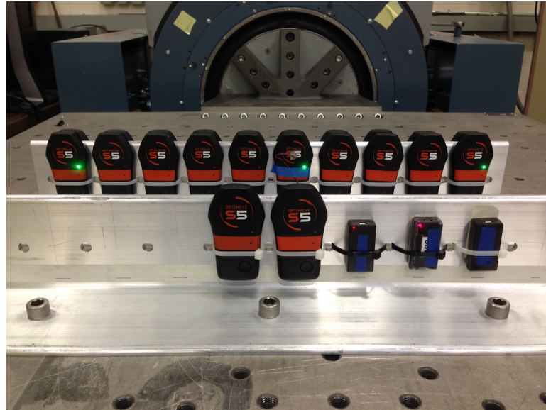
Fig 1. Accelerometer mounting bracket and shaker table configuration. The shaker table motion is in the fore-aft direction in this photo. As attached, the devices are subjected to motion in the X direction (front-back). The mounting bracket is rotated 90 degrees on the shaker table for Y direction motion (side-side). For Z direction motion, the table is removed, the drive motor is rotated 90 degrees, and the mounting bracket is attached directly to the drive motor output mount.
