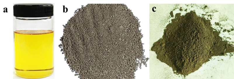
Figure 2. Products of vacuum distillation: (a) recycled oil, (b) recovered solid, and (c) PF-ECOSEAL.
