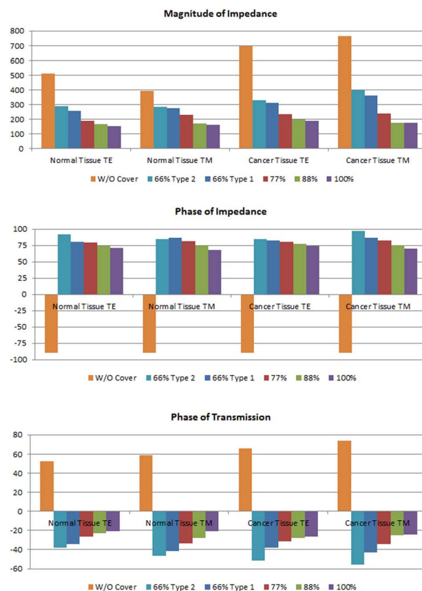
Fig. 9 Comparison of the effect of the core-shell nanoparticle filling factor on (a) magnitude of impedance, (b) phase of impedance and (c) transmission phase for normal and cancer tissues in TE and TM modes.
