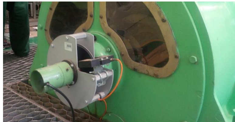
Figure 3. ETNP-10 laser heads are mounted on both free ends of the shaft and track the movement of perforated discs with 180 symmetrical slots along their perimeter ((a)—view from the engine side, (b)—view from the generator side).
