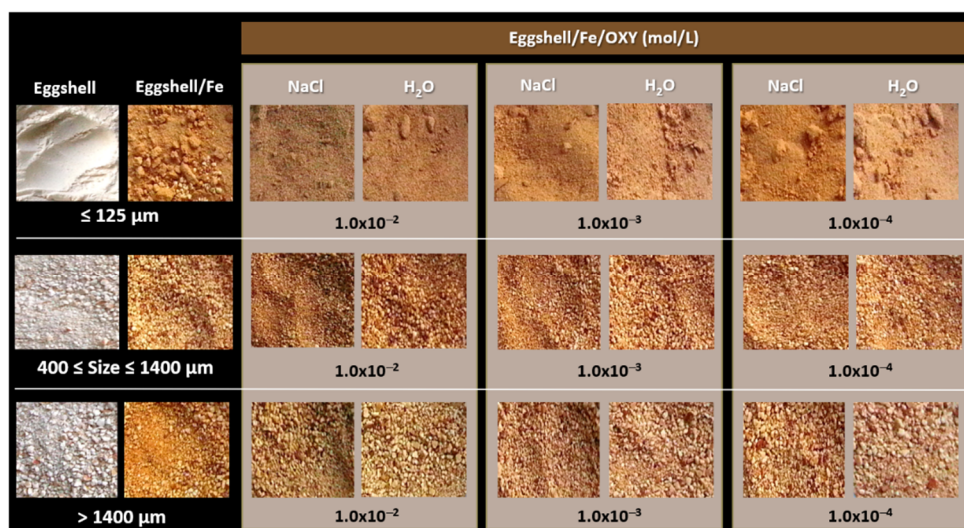
Figure 2. Pictures of the iron-modified eggshell materials, of different particle sizes, having previous incubation in water or NaCl, and undergoing reaction with antibiotic of concentrations ranging from 1.0 \times 10^{-4} to 1.0 \times 10^{-6} mol/L.
