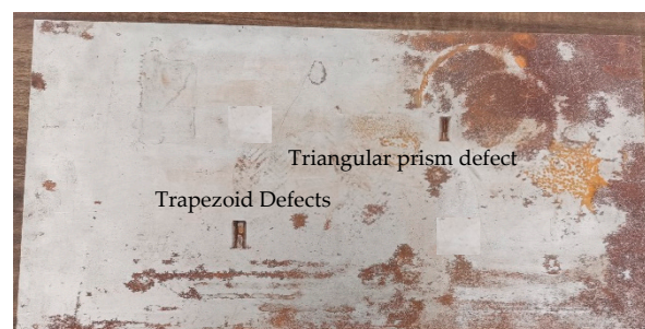
Figure 16. Schematic diagram of metal surface holding defects.
