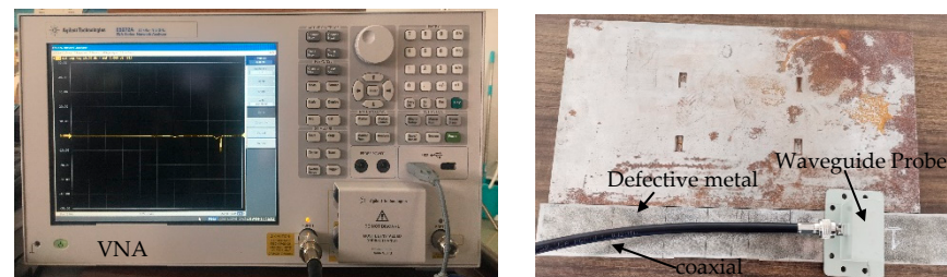
Figure 13. Schematic diagram of metal surface defect detection experiment.
