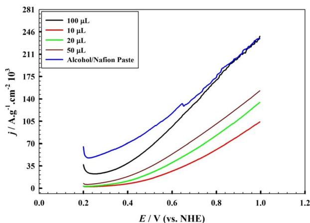
Fig. 6 Effect of the amount of catalyst (AFS-Cu-P) applied for the modification of the GC electrode. LSV with scan rate 10  $\text{mV s}^{-1}$  in 0.33 M hydrazine/1.0 M KOH.
