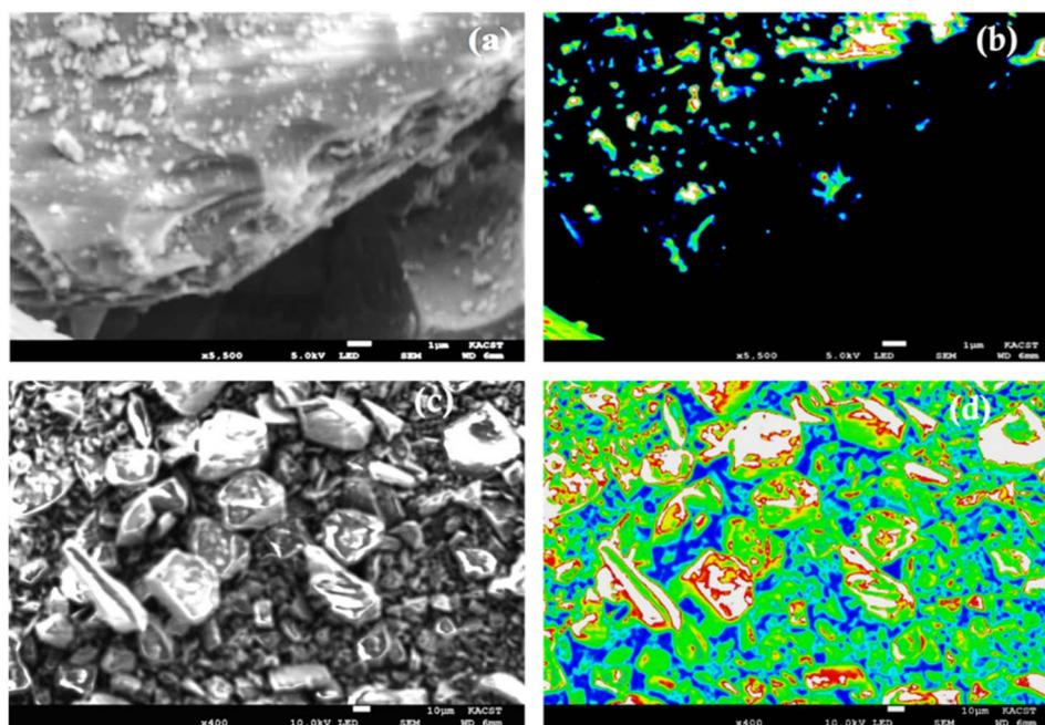
Fig. 2 (a) Surface morphology showing SiO<sub>2</sub> plates covered with nanostructured Cu particles for AFS-Cu-P. (b) Backscattering phase mapping of the Cu nanoparticle inclusion on the surface of the SiO<sub>2</sub> plates. (c) SEM image of the general distribution of the catalyst over the surface. (d) Phase mapping showing the different regions containing silicon and copper on the surface.
