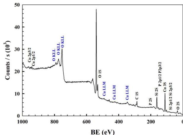
Fig. 3 XPS of the as-prepared AFS-Cu-P catalyst.
