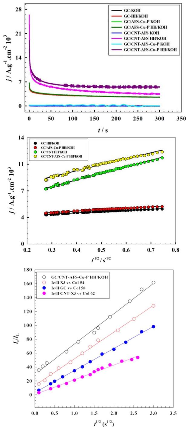
Fig. 9 (a) Chronoamperometry measurements over different electrodes in 1.0 M KOH and 0.33 M hydrazine/1.0 M KOH. (b) Relationship between catalytic specific oxidation current densities ( $j$ ) versus  $t^{-1/2}$  for different electrodes in 0.33 M hydrazine/1.0 M KOH. (c) Relationship between catalytic specific oxidation current density ratio versus  $t^{1/2}$  for different electrodes in the presence and absence of 0.33 M hydrazine/1.0 M KOH.
