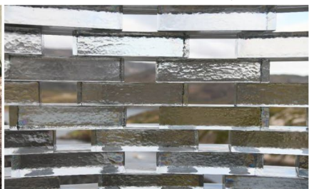
9. Top view of bonded bricks with the Fast-curing experimental Dowsil Adhesive (left) and 3M DP610 (right).
