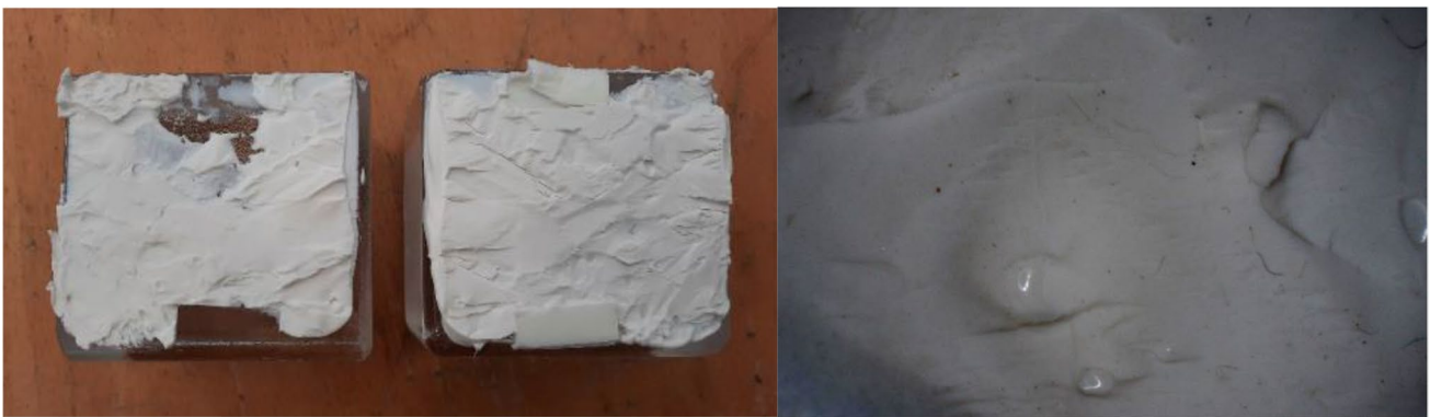
Fig. 15 Samples bonded with adhesive B presented either cohesive-adhesive or cohesive failure. The figure on the right shows such a zone of mixed failure, as observed with a Keyence VHX-7000 digital microscope
