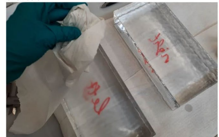
6. Bricks are removed and cleaned using isopropanol
