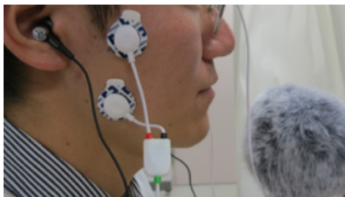
Figure 5. Experimental setup of the EMG probes, binaural microphones, and sound recorder with a windproof bore. EMG, electromyography.
