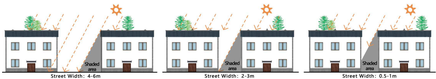
Fig 16. The influence of building height on microclimate in courtyard space.
