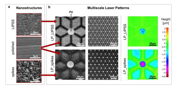
**Figure 1.** Nanostructures (LIPSS or spikes) and multiscale laser patterns (LP) produced by a femtosecond laser. (a) Scanning electron microscope (SEM) micrographs of polished surfaces and laser-nanostructured surfaces with LIPSS or spikes (tilt 45°). (b) SEM micrographs and focus variation microscopy of laser-patterned surfaces. LP\_LIPSS and LP\_spikes with a mix of polished and nanostructured areas. The micro-pits located in the center of the patterns were deeper and covered with LIPSS.
