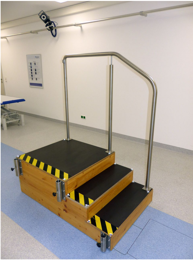
Fig. 2 Custom-made stairway scaffold with handrail for biomechanical stair climb analysis
