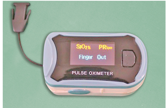
Fig. 4: Finger pulse oximeter (Choicemmed MD300C15D Pulse Oximeter, India) for measurement of pulse rate and oxygen saturation
