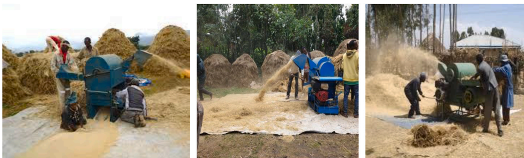
Fig. 11. Mechanized threshing machines of Teff in operation [52].
