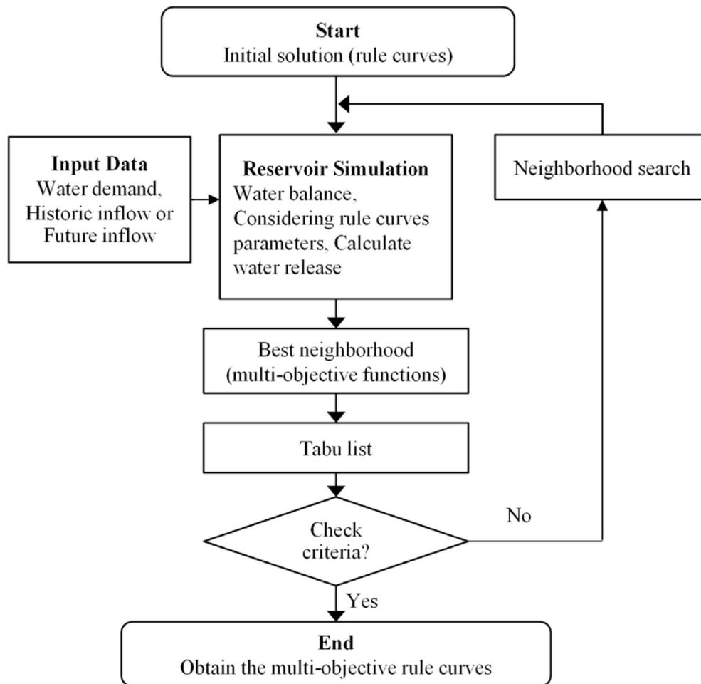
Fig. 2. Conditional tabu search algorithm connecting reservoir simulation for searching rule curves.
