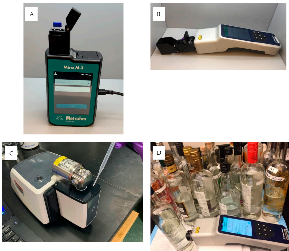
Figure 1. Vibrational spectroscopy units used in this research. (A) Metrohm Mira M3 (785 nm) Raman instrument, (B) handheld Progeny Rigaku (1064 nm), (C) portable Agilent Cary 630 FT-IR device, and (D) handheld Progeny Rigaku (1064 nm) instrument conducting the through-the-bottle analysis.
